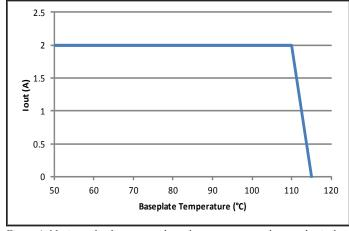
Figure 4: Maximum load current vs. baseplate temperature when conductively cooled. Note: The system design must provide a suitable thermal path that maintains the baseplate temperature below 100 °C.
