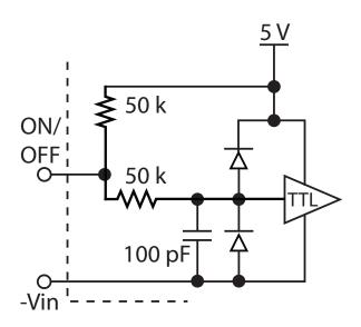
Figure B: Internal ON/OFF pin circuitry
