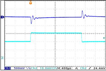
Figure 5: Output voltage response to step-change in load current (50%-75%-50% of lout(max);  $dI/dt = 0.1A/\mu s$ ). Load cap:  $1 \mu F$  ceramic and  $15 \mu F$  tantalum capacitors. Ch 1: Vout, Ch 2: Iout (1A/div).
