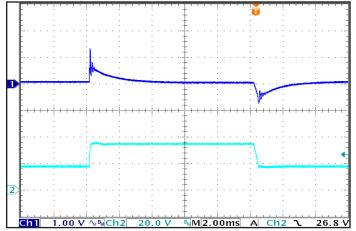
Figure 6: Output voltage response to step-change in input voltage (250 V/ms, Vnom-Vmax-Vnom). Load cap: 1 µF ceramic capacitor. Ch 1: Vout, Ch 2: Vin.
