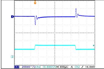
Figure 5: Output voltage response to step-change in load current (50%-75%-50% of lout(max);  $dI/dt = 0.1 \ A/\mu s$ ). Load cap:  $1 \ \mu F$  ceramic and  $15 \ \mu F$  tantalum capacitors. Ch 1: Vout, Ch 2: lout (5A/div).
