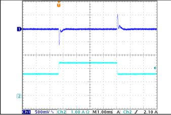
Figure 5: Output voltage response to step-change in load current (50%-75%-50% of lout(max);  $dI/dt = 0.1A/\mu s$ ). Load cap:  $1 \mu F$  ceramic and  $15 \mu F$  tantalum capacitors. Ch 1: Vout, Ch 2: lout (1A/div).
